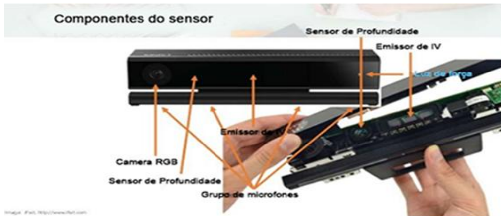
Figura 2.5 – Componentes do sensor Kinect, adaptado de (KERKHOVE, 2014)
