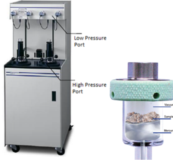
Figure 2.3: AutoPore IV Series Mercury Porosimeter (left) and glass penetrometer (right) used in automated MICP acquisitions.
