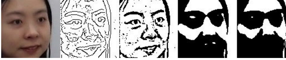
Figure 2.4: Preprocessings: (a) original image [3]; (b) Canny filter; (c) Adaptive Gaussian filter; (d) Sauvola binarization; (e) Otsu binarization.
