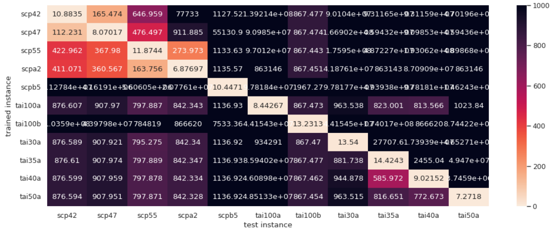
Figure B.7: RMSE_{AVG} for random forest regressors, trained using features ( iteration , cost , best_cost ), when evaluated on datasets from different instances and problems.
