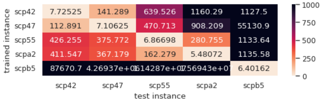
Figure 4.5: RMSE_{AVG} for random forest regressors, trained on SCP instances using features ( best\_cost , best ), when evaluated on datasets from other SCP instances.
