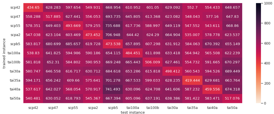
Figure 4.14: RMSE_{AVG} for XGBoost regressors, trained using features ( iteration , iterations_since_last_min , iterations_since_best_cost , total_single_mins_found ), when evaluated on datasets from different instances and problems.
