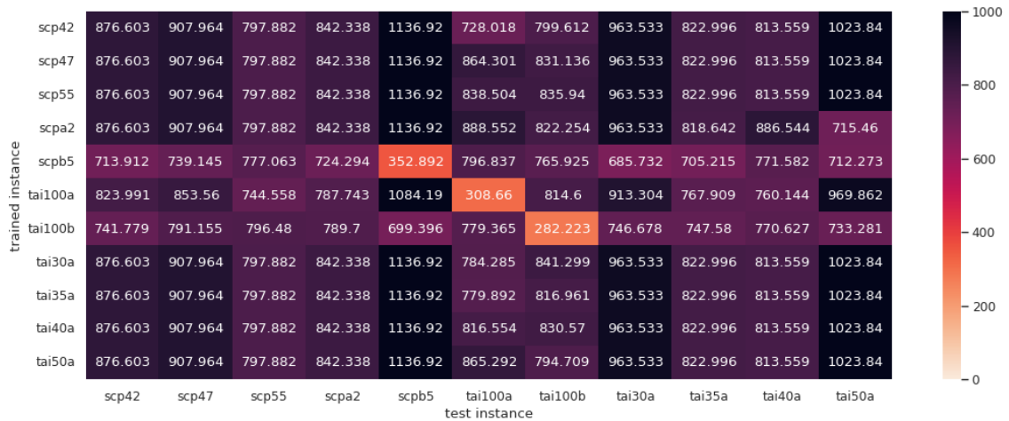
Figure B.13: RMSE_{AVG} for XGBoost regressors, trained using features ( iteration , cost , best ), when evaluated on datasets from different instances and problems.
