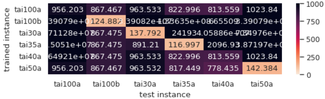
Figure 4.9: RMSE_{AVG} for XGBoost regressors, trained on QAP instances using features ( best\_cost , best ), when evaluated on datasets from other QAP instances.
