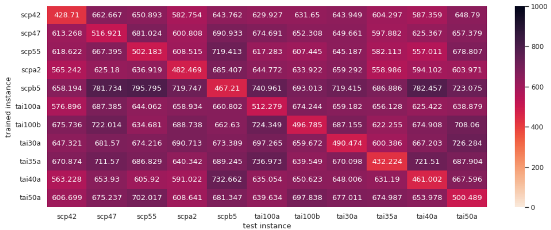
Figure B.5: RMSE_{AVG} for decision tree regressors, trained using features ( iteration , iterations\_since\_last\_min , iterations\_since\_best\_cost , total\_single\_mins\_found ), when evaluated on datasets from different instances and problems.
