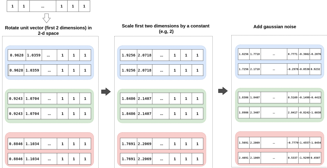
Figure 4.2: Generation of the initial embedding ( h_0 ) step by step. Example with three groups of nodes, represented by the colors blue, green, and red.
