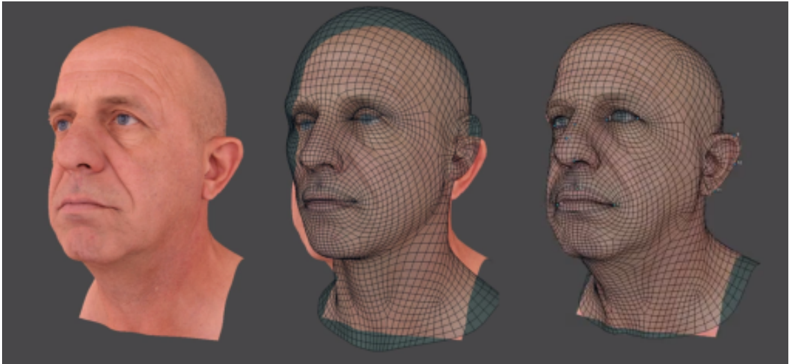
Figure 2.4: A template mesh being warped to another head model.
