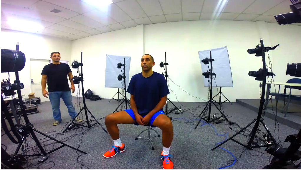
Figure 2.1: Photogrammetry Rig with 20 Canon EOS T5i cameras. The subject was a professional volleyball player from the Brazilian team.
