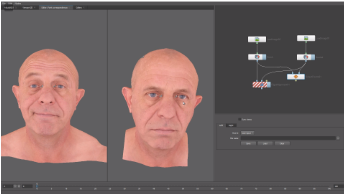
Figure 2.3: R3DS Wrap interface. Two models being aligned as well as a few correspondence points for the rigid alignment process. On the right corner the nodes used for loading meshes and textures aside from nodes to apply rigid alignment and set correspondence points.
