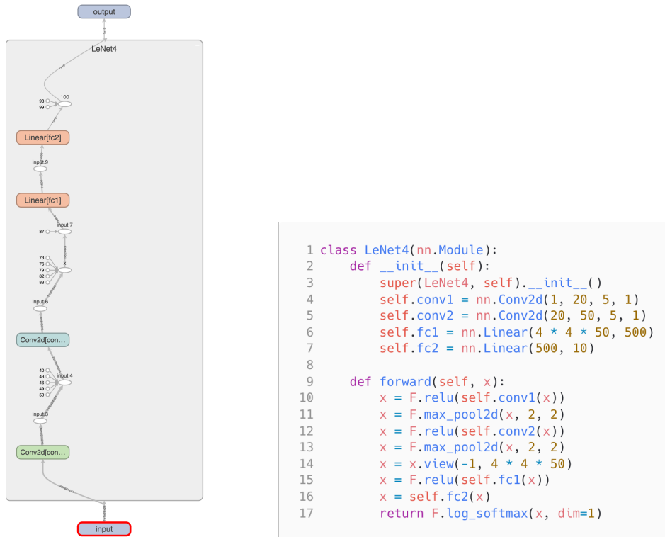
Figure 3.1: LeNet-4 example of PyTorch computational graph (left panel) and the required code to implement it (right panel).
